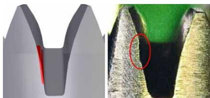
*The defective spot (left) becomes visible in the gear (right).*
