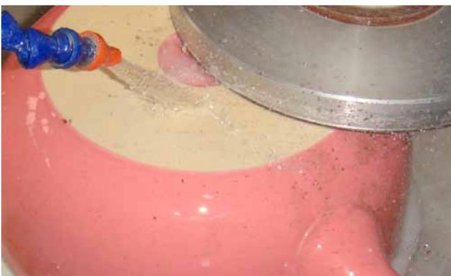
*Grinding process for the fondue pots made of ceramic*
